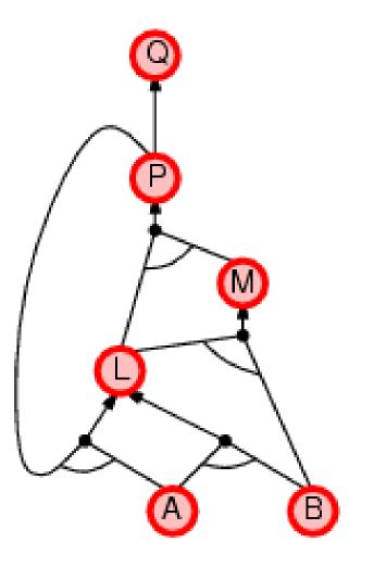
$\begin{array}{l} P \Rightarrow Q \\ L \wedge M \Rightarrow P \\ B \wedge L \Rightarrow M \\ A \wedge P \Rightarrow L \\ A \wedge B \Rightarrow L \\ A \end{array}$
